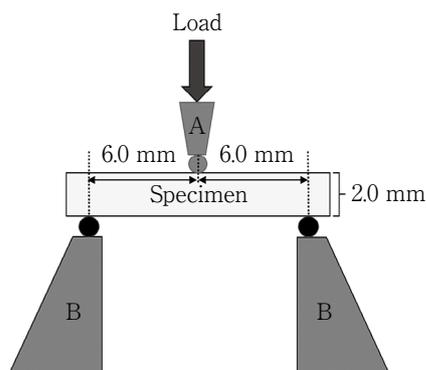
**Fig. 3** Schematic diagram of the three-point bending test (head speed : 1.0 mm/min)
