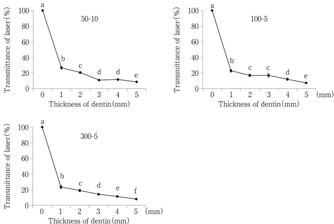
**Fig. 3** Transmittance of Nd: YAG laser for different dentin thicknesses
