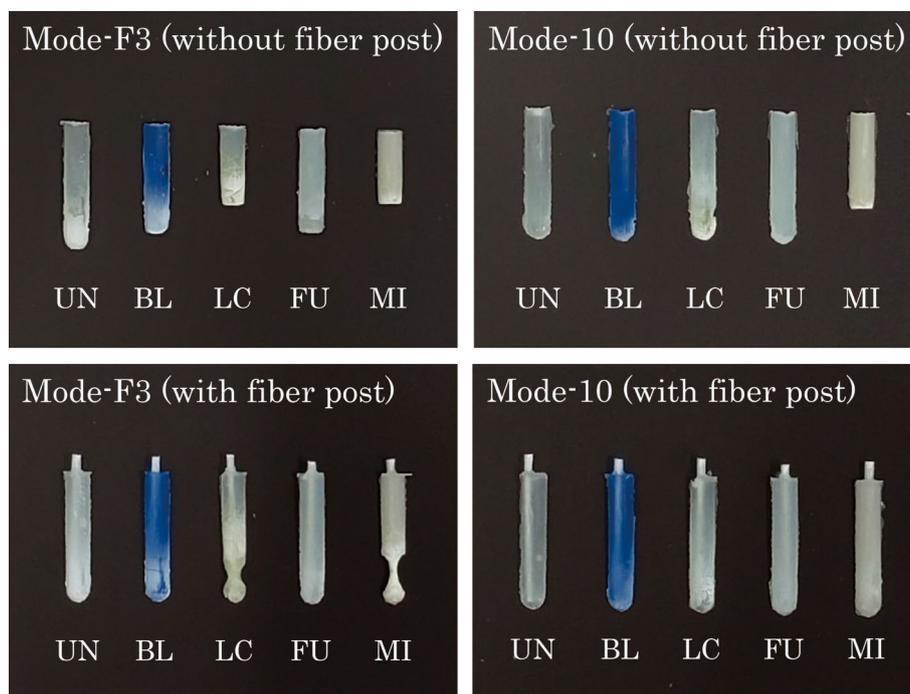
**Fig. 2** Representative images of polymerization resins after acetone washing
