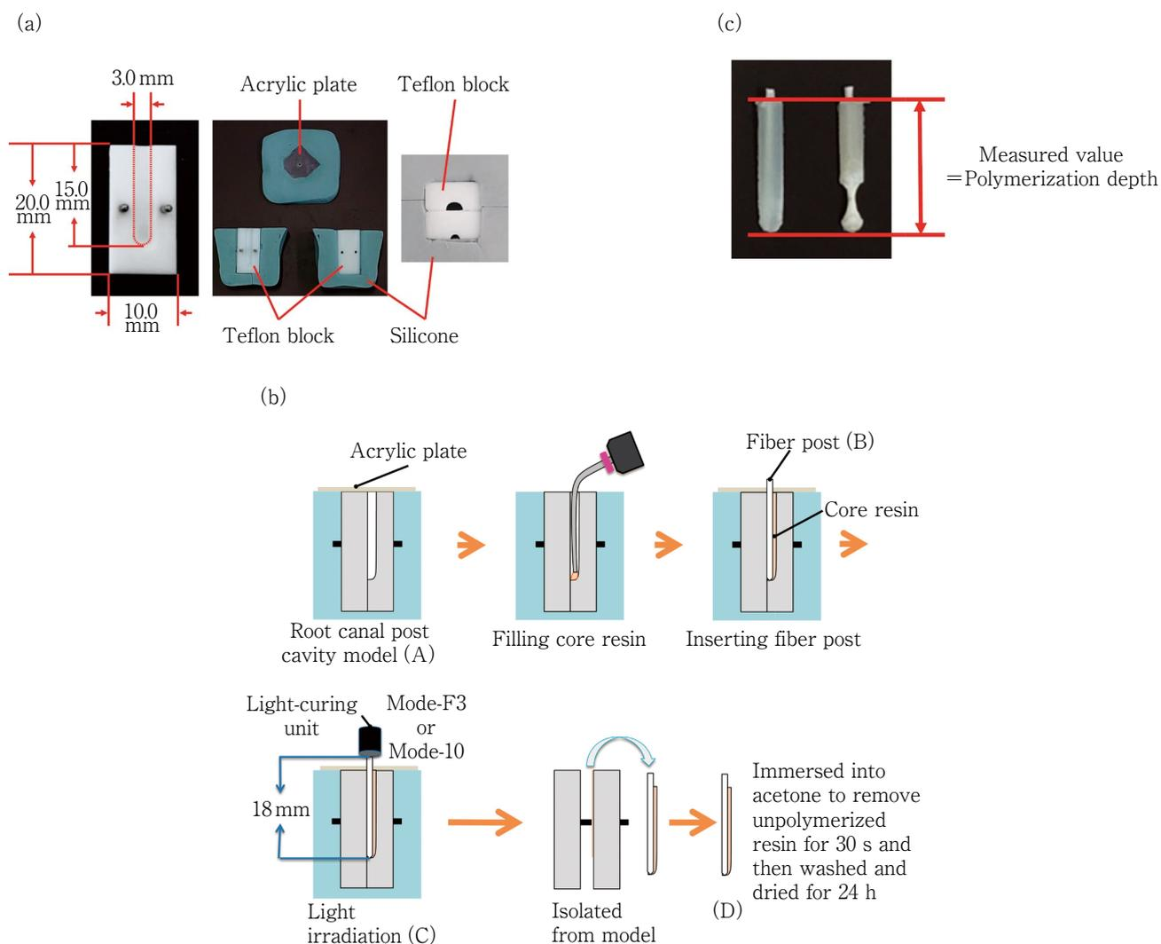
**Fig. 1** Experimental system for polymerization ratio and depth measurement
