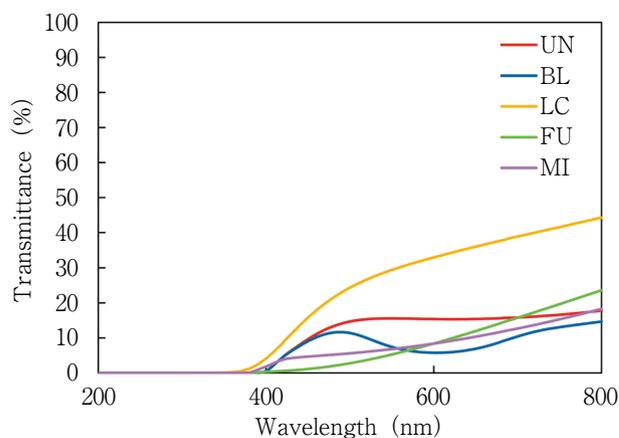
**Fig. 3** Transmission spectra of each polymerization resin
