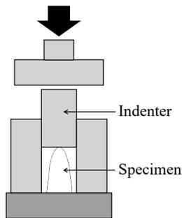
**Fig. 5** Schematic diagram of static load test (head speed : 1.0 mm/min)
