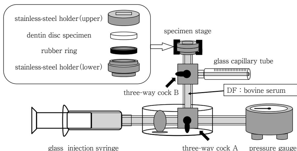
**Fig. 2** Schematic diagram of a dentin hypersensitivity model
