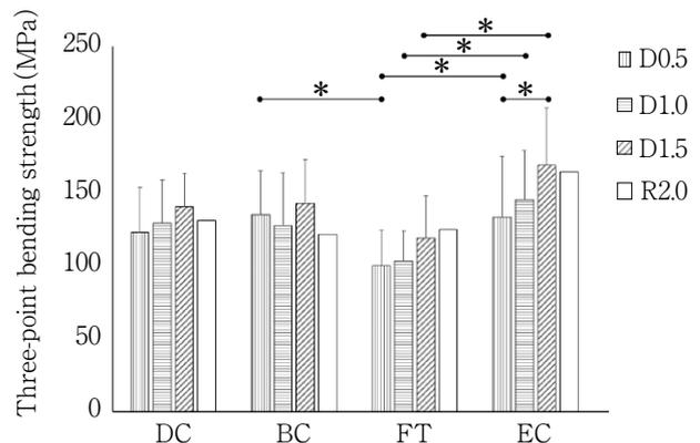
**Fig. 6** Measured values of three-point bending strength for each group (\* :  $p < 0.05$ ,  $n = 14$ )
