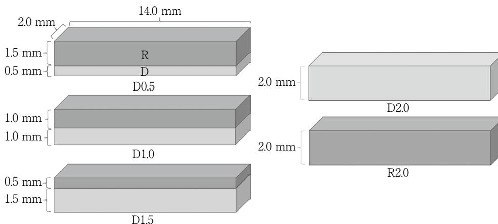
**Fig. 2** Schematic diagram of each plate specimen
