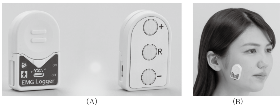
Fig. 1 The wearable electromyography (EMG) device (EMG Logger) used in this study (A) The appearance of the device, showing the main unit and the electrode surface. (B) The device attached to the masseter muscle region of a subject for measurement.
